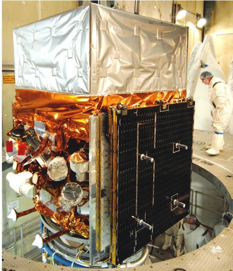
Figure 4.8.: The *Fermi* Gamma-ray Space Telescope shortly before launch with the Large Area Telescope at the top, and the Gamma-ray Burst Monitor at the left bottom side of the instrument. The solar panels are folded at the side. (NASA, DOE)
