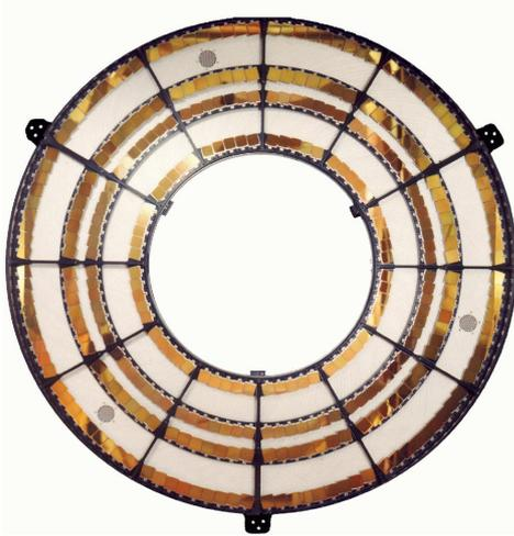
**Figure 5.4:** HETG facets mounted on the Rowland torus (from [http://space.mit.edu/HETG/hetg\\_info.html](http://space.mit.edu/HETG/hetg_info.html)).
