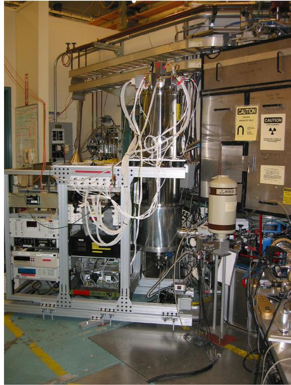
**Figure 4.8:** EBIT Calorimeter Spectrometer (ECS) installed at EBIT-I in Livermore (from <https://ebit.llnl.gov/EBITPhotoGallery.html>).
