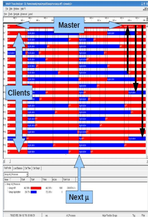
Figure 24: Screenshot of the output of *Traceanalyzer*. The blue and red bars indicate that the corresponding clients are working or idle respectively.
