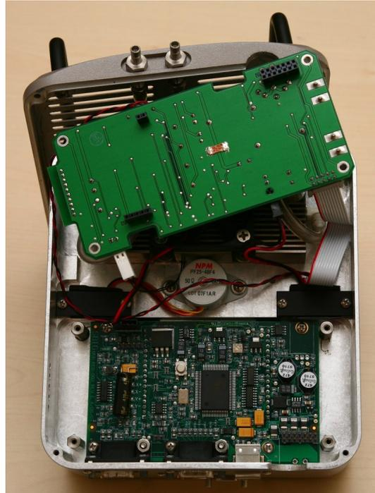
Figure 3.3: Disassembly of the STL-11000 showing the EZ-USB AN2131 in the center
