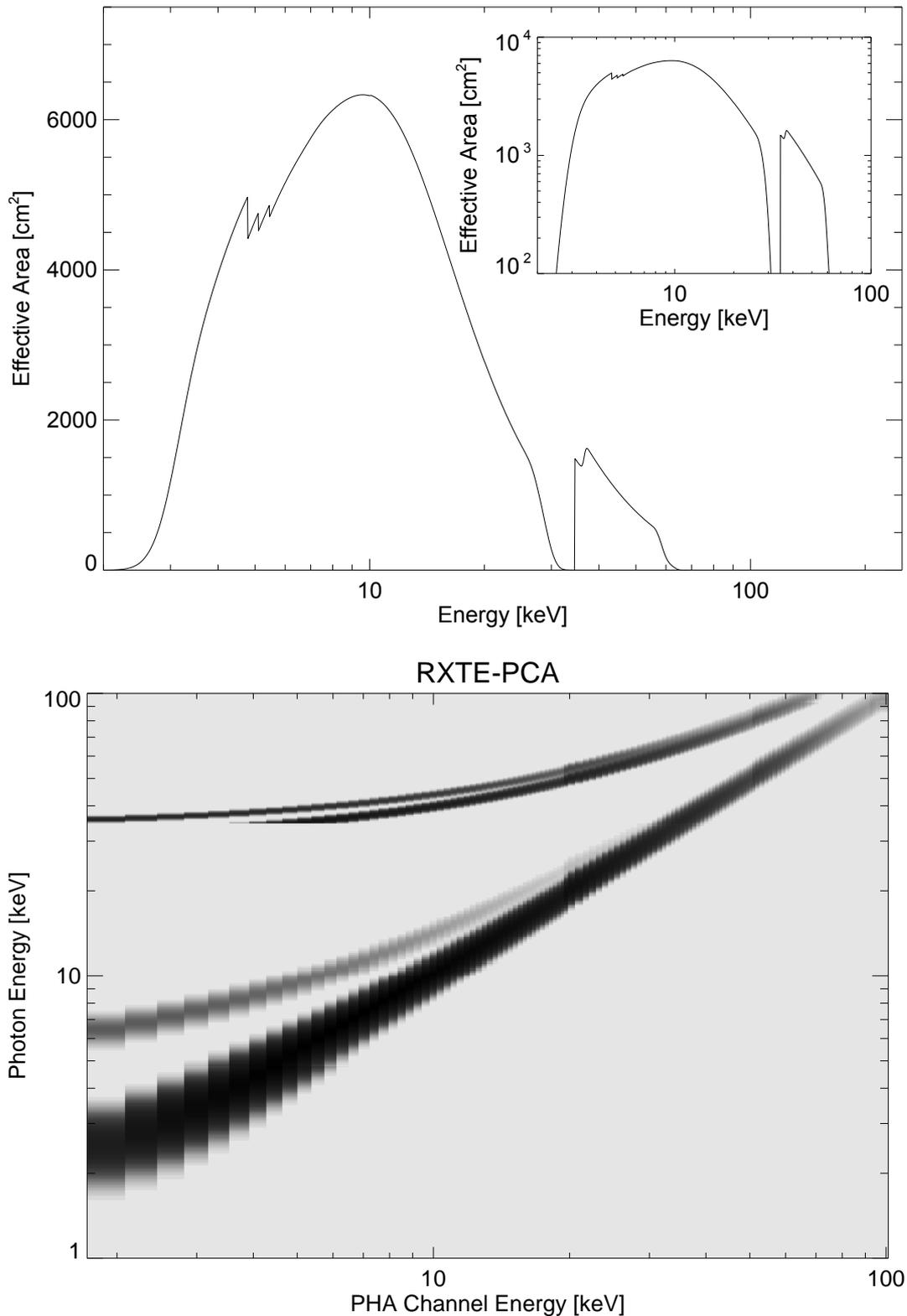
Figure 5.1: The top panel shows the PCA effective area as a function of energy. In the inset, the same data are plotted in logarithmic form. The effective area is the main component of the ARF. (Wilms, 1998, Fig. 4.3) The bottom panel contains PCA's response matrix. The gray scale illustrates the probability, that a photon of a given energy is registered in a certain PHA-channel. (Ingo Kreykenbohm, priv. comm.)
