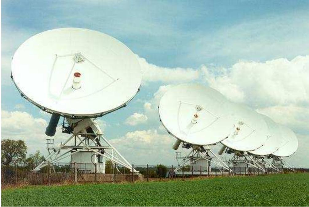
Figure 2.7: The Ryle telescope in Great Britain. The antennas can be moved on rail tracks. The array consists of eight telescopes. Five of them are in a compact configuration here, as the photo was taken. ([www.mrao.cam.ac.uk/telescopes/ryle/](http://www.mrao.cam.ac.uk/telescopes/ryle/))
