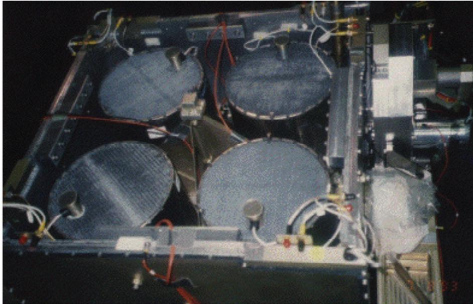
Figure 2.5: The four scintillation counters of one of HEXTE's clusters. There are two of these instrument aboard the satellite. ([http://heasarc.gsfc.nasa.gov/docs/xte/learning\\_center/hexte.html](http://heasarc.gsfc.nasa.gov/docs/xte/learning_center/hexte.html))
