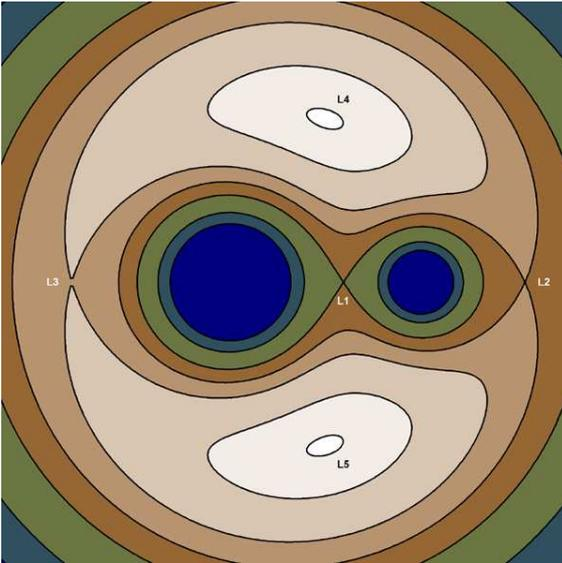
Figure 3.2: Visualization of the gravitational potential  $\Phi(\vec{r})$  of a binary system. The five Lagrangian points  $L_1$  to  $L_5$ , where  $d\Phi(\vec{r})/d\vec{r} = 0$ , are shown in this figure. (source: <http://members.wri.com/jeffb/visualization/lagrange.shtml>)
