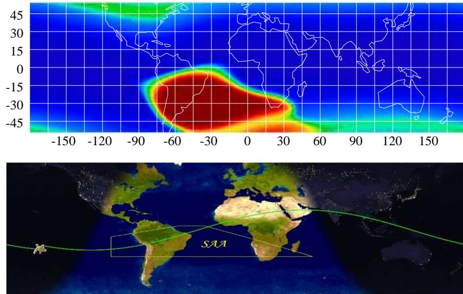
Figure 2.2: The picture on the top shows the location of the South Atlantic Anomaly as measured by *ROSAT*. (Kreykenbohm, 2004) *RXTE* has a smaller inclination and does not pass completely through this region. Below a schematic map of *RXTE*'s orbit. The theoretical position of the SAA, where the satellite is not able to operate, is indicated in the picture. (The picture can be found at <http://heasarc.gsfc.nasa.gov/docs/xte/SOF/CurrentLocation3.html>)
