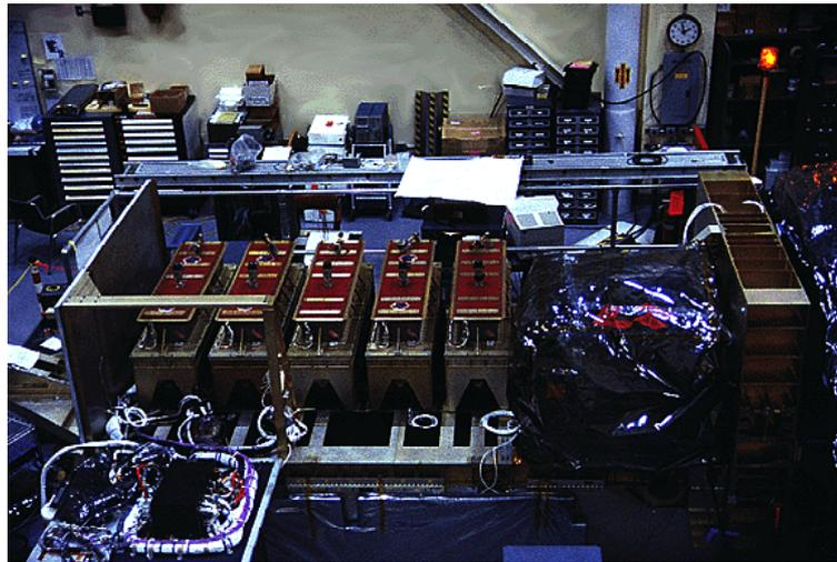
Figure 2.3: A view of *RXTE*'s assembly. Clearly visible are the five nearly identical proportional counter units (PCUs) of the proportional counter array in the body of the spacecraft. (<http://science.hq.nasa.gov/kids/imagers/ems/xrays.html>)
