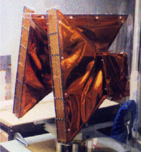
Figure 2.6: The three shadow cameras on the ASM. A position-sensitive proportional counter is located at the small end of each part, which detects the photons passing through the coded-mask on the top. ([http://heasarc.gsfc.nasa.gov/docs/xte/learning\\_center/asm.html](http://heasarc.gsfc.nasa.gov/docs/xte/learning_center/asm.html))
