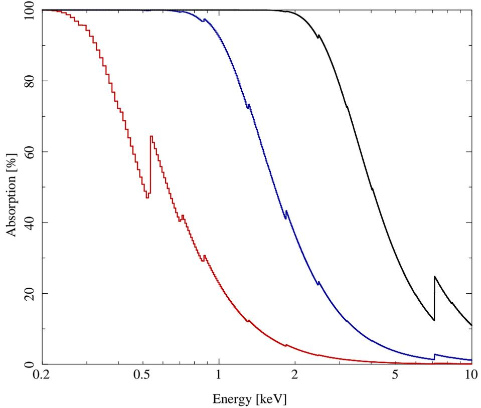
Figure 5.2: Plot of the photoelectric absorption modeled with the `phabs` function. The colors stand for different values of the equivalent hydrogen column  $N_{\text{H}}$  in units of  $10^{22}$  atoms/cm<sup>2</sup>. For the red graph a  $N_{\text{H}}$  of 0.1 was used, 1 for the blue one, and 10 for the black one. Values for Cy X-1 lie between 0.1 and 1. Therefore, one can see, that the PCA data above 5 keV, which was used for spectral fitting, is only marginally affected.
